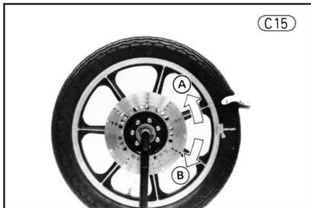
A. Use heavier weight. B. Use lighter weight.
