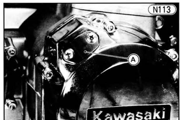
A. Inspection Window Cover
